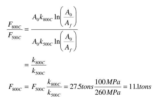
Thus a press with a capacity of at least 27.4 tons is needed to extrude the bar at 500C, whereas a press with only a capacity of 11.1 tons is needed to extrude the bar at 800C.
