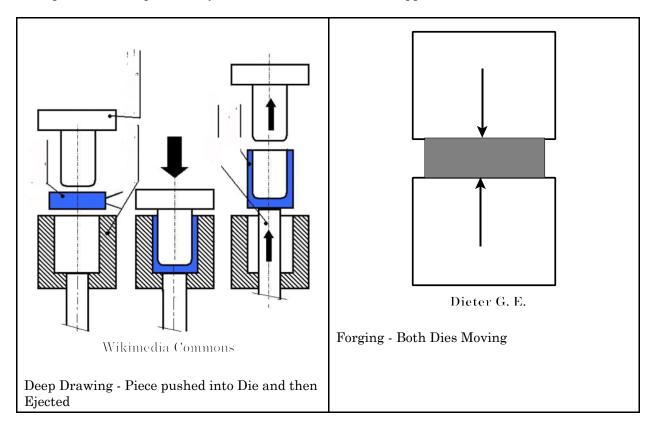
4) During the sheet metal practica you made a bowl. Describe what you did using proper terminology. Would it be possible to make the same bowl using a steel alloy with an ultimate tensile strength of 50ksi and a yield strength of 30ksi? Assume the sheet was 0.010" thick and that the disk was 4.00" in diameter.
